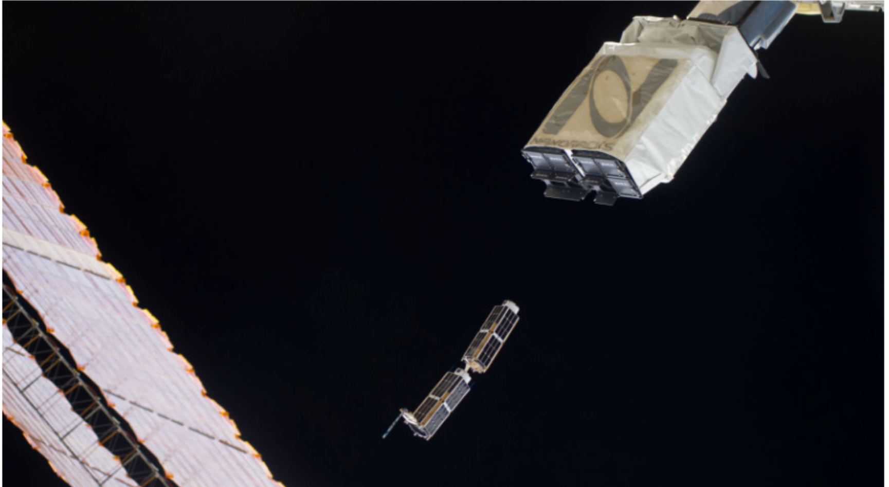
A3R and Centennial-1 (the shorter cubesat) deploy from the NanoRacks dispenser aboard ISS. Credit: NASA
